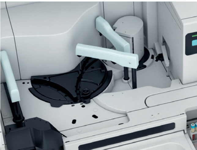
CS-5100 uses three reagent arms, out of which one arm is dedicated to Thrombin reagent to avoid contamination and minimise the risk of carry-over.
