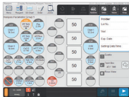
Figure 3 Reagent management screen. You can easily check the remaining volume of reagent, the remaining number of tests, on-board stability time and other information.
